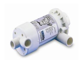
The Bait Sentry Livewell Pumps are designed for easy installation and trouble-free operation. Magnetic Drive technology eliminates unnecessary failures. Motors keep running after ingesting debris or even when running dry. Patented antairlock feature allows the pump to clear trapped air in rough water or when boat is anchored. Includes dual port for easy washdown pump connection.
