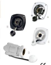
The Shurflo exclusive diaphragm design prevents high-pressure damage often caused by city water systems. These high performance water entries limit water pressure and they include a check valve. 3/4" (19mm) GSH Female swivel inlet. 1/2" (13mm) NPSM - Male Outlet
