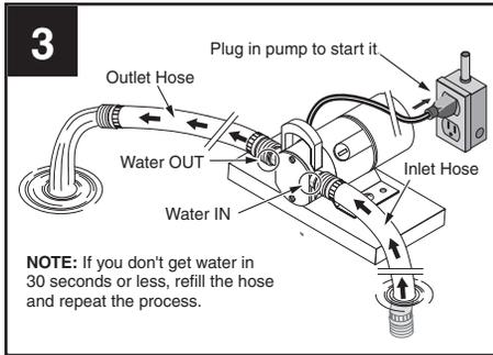
**INLET HOSE GOES IN THE WATER; OUTLET HOSE STAYS OUT OF THE WATER. MOTOR MUST STAY DRY**
