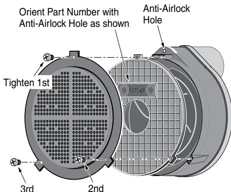
Install shield and tighten screws in sequence as shown.
