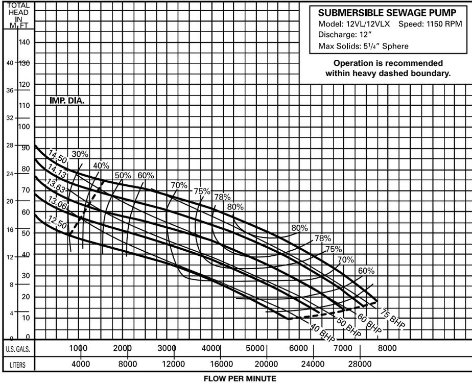
Pump performance is based on clear water (1.0 specific gravity @ 68°F) and pump fluid end (hydraulic) efficiency. Motor data based on 40°C ambient temperature.
