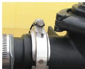
Captured nut and bolt design reduces assembly and maintenance time by eliminating the need to feed a track through the worm gear.
