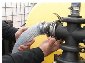
Clamshell design holds fittings in place before tightening the bolt for easy assembly. The worm gear clamps need to be engaged before being capable of holding fittings in alignment.
