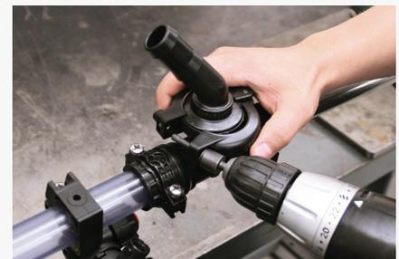
The clamshell and captured bolt and nut designs of Hypro Universal Flange Clamp improves productivity by reducing assembly time and eliminating joint leaks.
