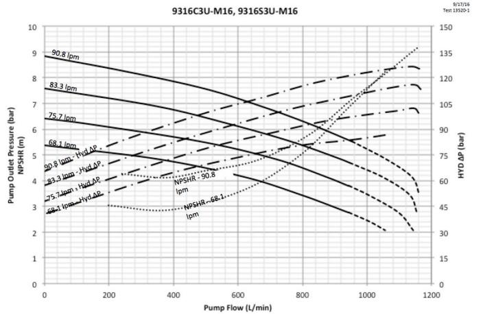
Note: The dashed portion of the pump curves is outside the recommended operating range, and can only be achieved with sufficient NPSHa. Refer to Installation Instructions.
