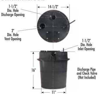
All dimensions in inches. Metric for international use. Component dimensions may vary ± 1/8 inch. Dimensional data not for construction purpose unless certified. Dimensions and weights are approximate. On/Off level adjustable.
