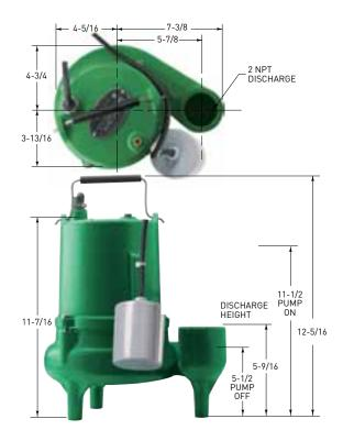
All dimensions in inches. Metric for international use. Component dimensions may vary  $\pm$  1/8 inch. Dimensional data not for construction purpose unless certified. Dimensions and weights are approximate. On/Off level adjustable.
