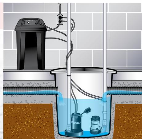
Includes: battery case control unit, 12V pump, reed switch, AC power supply, wireless gateway, 1-1/4" NPT to 1-1/2" glue PVC elbow
