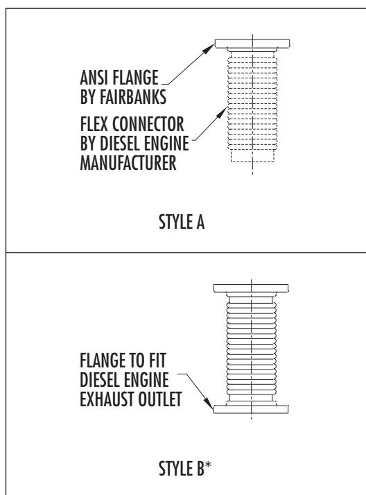
\*FLANGED FLEX CONNECTOR PROVIDED BY DIESEL ENGINE MANUFACTURER. NO ADDITIONAL FLEX CONNECTOR OR ADAPTOR FITTING IS REQUIRED OR PROVIDED BY FAIRBANKS NIJHUIS™.
