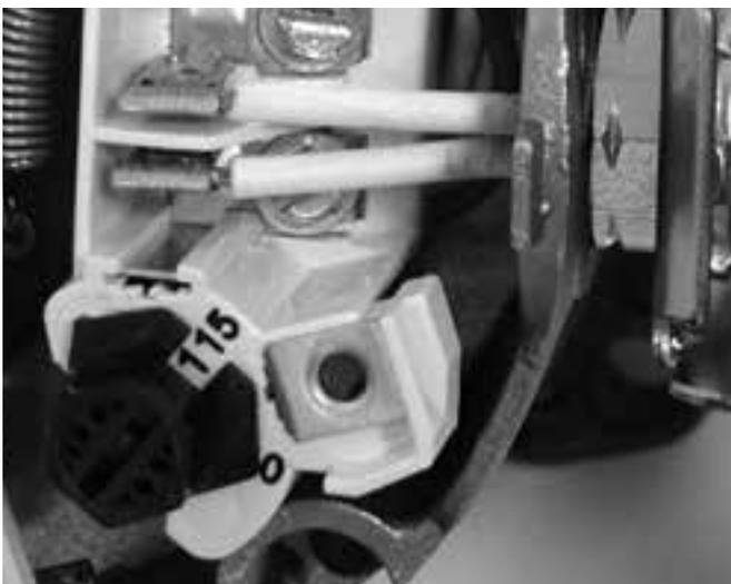
**Figure 4: Motor Set for 115 Volt Operation**
