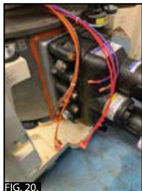
21. Connect the Thermistor sensor and High Limit Switch.
