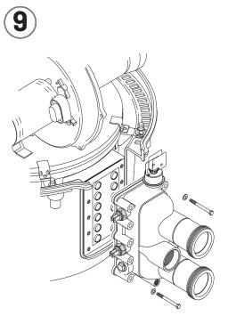
Carefully remove the MANIFOLD and ADAPTER.
