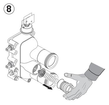
Carefully remove the spring-loaded thermal regulator.
