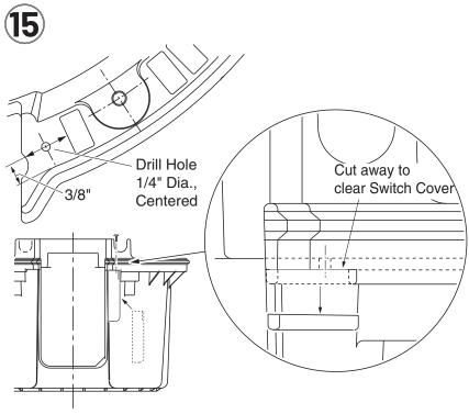
Install the second switch cover as shown when retrofitting a new manifold.
