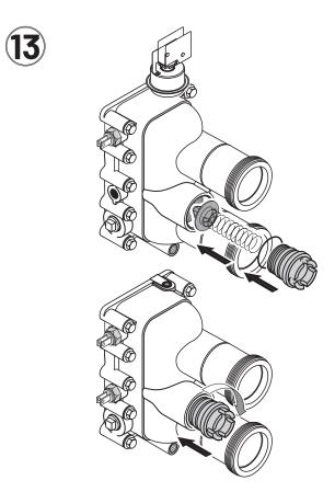
Install the Thermal Regulator in the Manifold.
