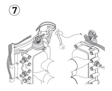
Remove the switch covers and disconnect the wires from the safety switches. The wires are color coded and marked for the switches they are connected to.
