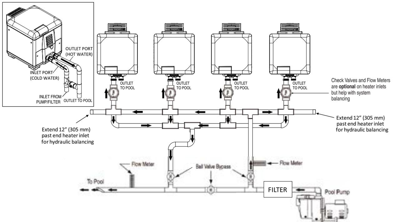
Figure 6. Four MasterTemp® 125 Heaters Plumbing Hydraulic Diagram
