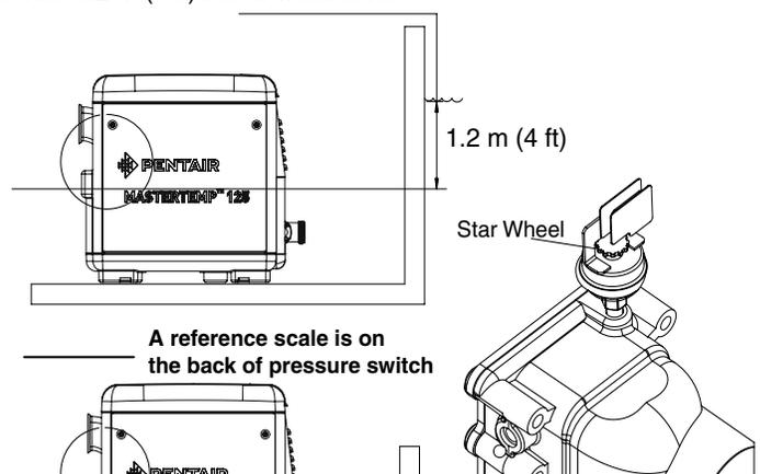
Turn star wheel **counterclockwise** to lower pressure set point if pressure switch is more than 1.5 m (5 ft) above water level
