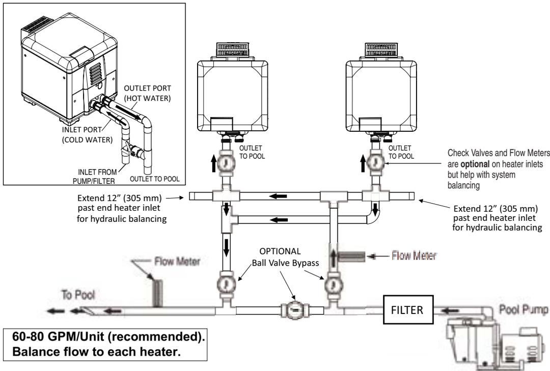
Figure 5. Two MasterTemp® 125 Heaters Plumbing Hydraulic Diagram
