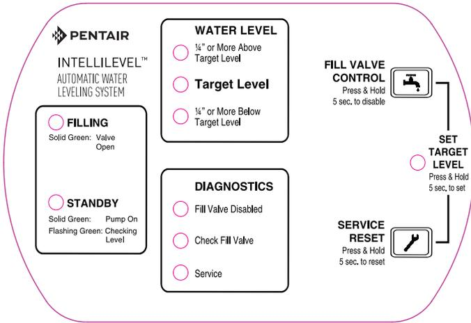
IntelliLevel™ Automatic Water Leveling System Control Pad
