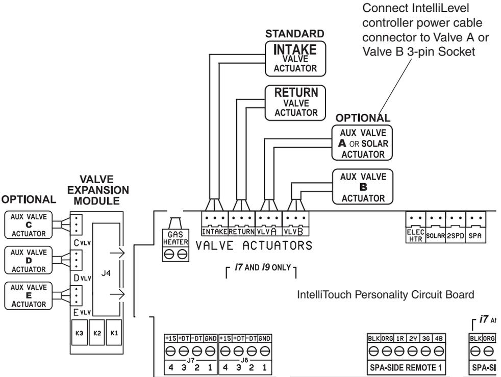
IntelliTouch Control System Circuit Board
