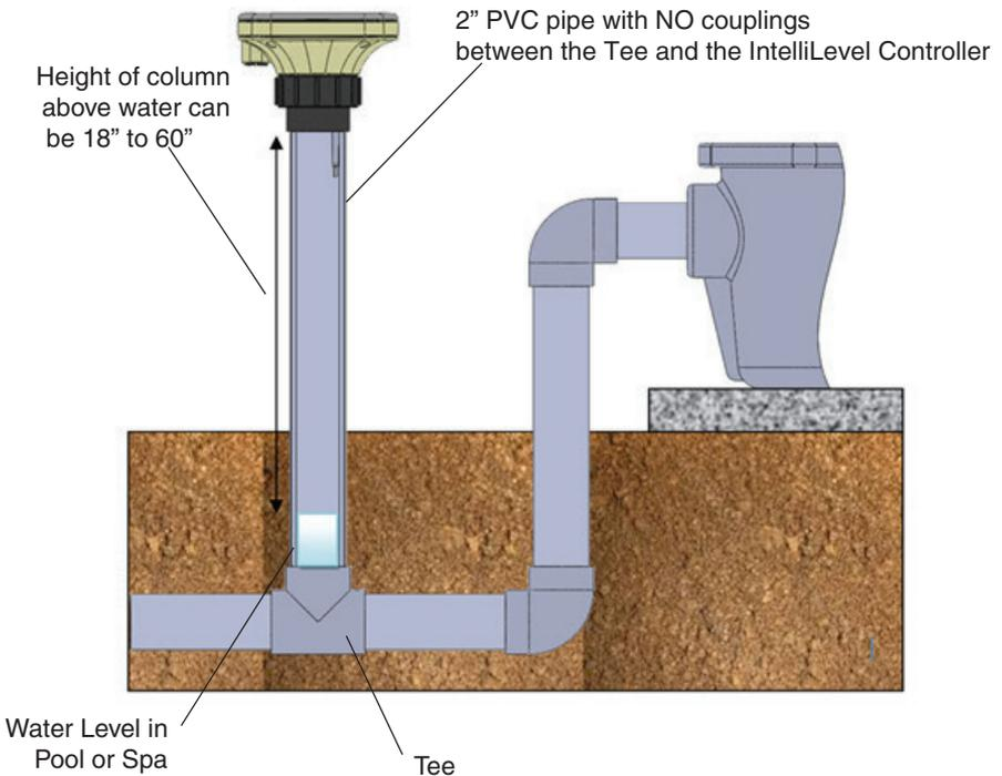
Main Drain Installation Diagram
