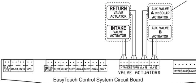
EasyTouch Control System Circuit Board
